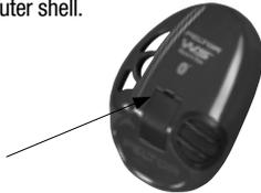
Insert a tool or finger under the edge of the clamp and pull it out 3–4 mm. Press/slide the clamp down. Remove the shell. Insert the rechargeable AAA NiMH batteries included with the product.
