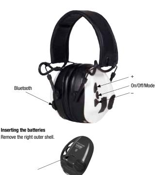
Insert a tool or finger under the edge of the clamp and pull it out 3–4 mm. Press/slide the clamp down. Remove the shell. Insert the rechargeable AAA NiMH batteries included with the product.
